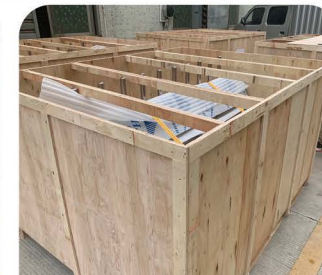
02 Fasten by belt and reinforce by beam
